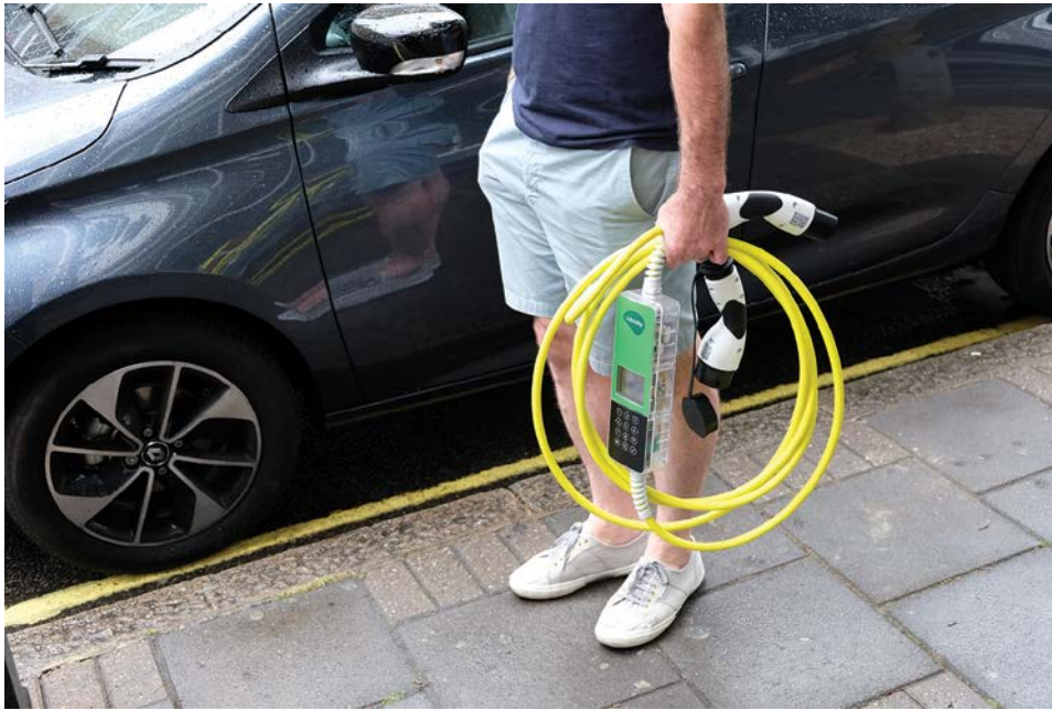
▼ Figure 5.7 Link cable incorporating a meter (courtesy of Ubitricity)
